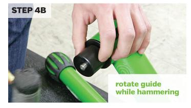
With the bushing plunger in place, insert the bushing plunger guide over the bushing plunger and into the left side of the quick release bushing.
