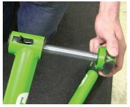
NOTE: if the threaded rod will not go through easily, tap handle lightly with the hammer to align it properlythen it should move freely.
